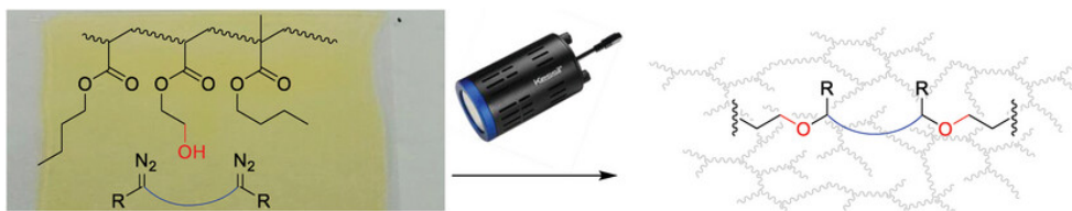
Figure 2. The acrylic crosslinking reaction presented in Chapter 3.
