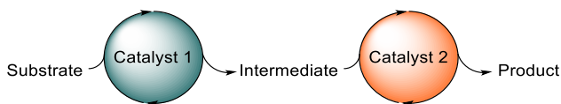
Figure 1: Orthogonal tandem catalysis scheme with 2 catalytic cycles. The substrate is converted by catalyst 1 to the intermediate, that is subsequently converted by catalyst 2 to form the final product.
