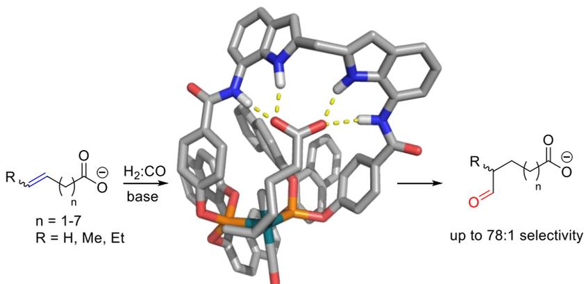
Scheme 1 Regioselective hydroformylation of internal and terminal unsaturated carboxylic acids *via* supramolecular substrate preorganization using RhDIMPhos complexes.
