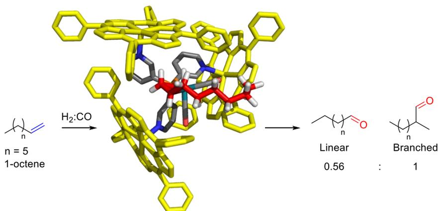
Scheme 2 Branched selective hydroformylation of 1-octene with [Rh(H)(CO)<sub>3</sub>(P(*m*Py<sub>3</sub>(ZnTPP)<sub>3</sub>))] (DFT modeled structure). ZnTPP building blocks depicted in yellow for clarity.
