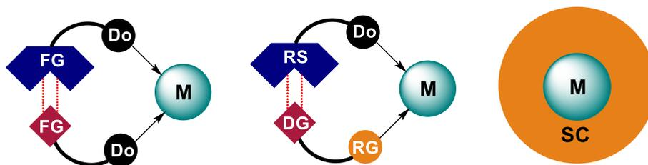
Figure 1 Supramolecular strategies commonly applied in the hydroformylation Left: supramolecular self-assembled bidentate ligands Middle: Supramolecular substrate preorganization, Right: Second coordination sphere catalysis. M = metal center, FG = Functional group, DG = directing group, RG = reactive group, RS = recognition site, Do = donor center, SC = Second coordination sphere
