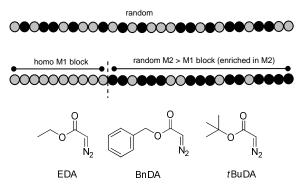
**Figure 1.** Schematic representation of random and poly({M1}<sub>b</sub>-{M2-*ran*-M1}<sub>b</sub>) block copolymers prepared from ethyl, benzyl and *t*-butyl diazoacetate.
